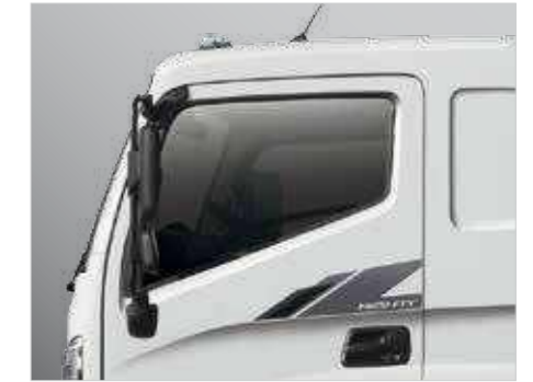
Taller, Wider Side Glass A taller, wider side window provides the driver with a much better view for safer driving.
